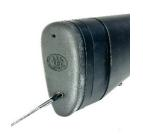
STEP 2: USING A 13MM SOCKET REMOVE THE LOCK NUT AND LOCK WASHER FROM FIREARM. THEN SLIDE THE BUTTSTOCK OFF OF THE THREADED ROD.
